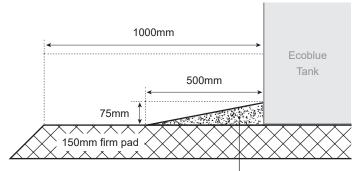
Concrete pad or blue metal aggregate
