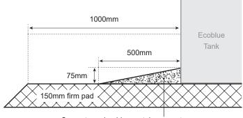
Concrete pad or blue metal aggregate
