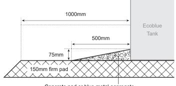
Concrete pad or blue metal aggregate
